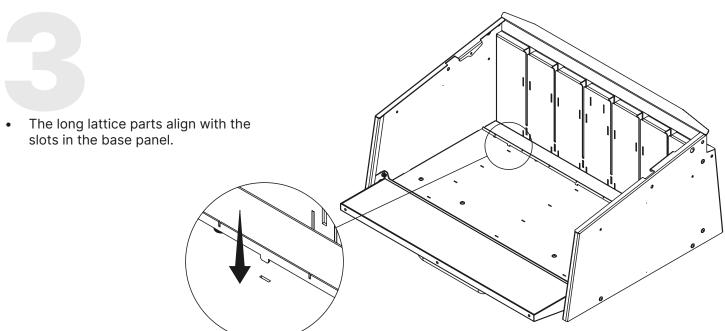
Position all long lattice parts by aligning with the slots in the base and pushing into position.
