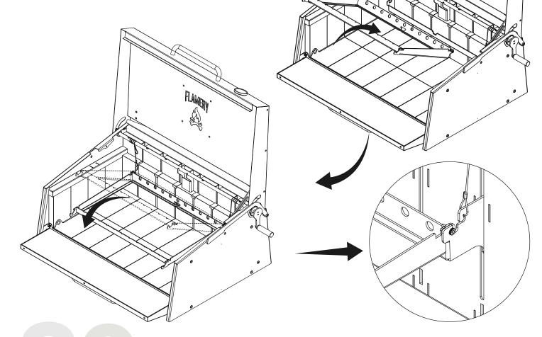
Using the Stainless Steel Grill Lock, lock the Grill Frame to the Grill Support by pushing the Grill Lock into the central slot in the frame, and allow it to sit against the bottom of the Grill Frame.
