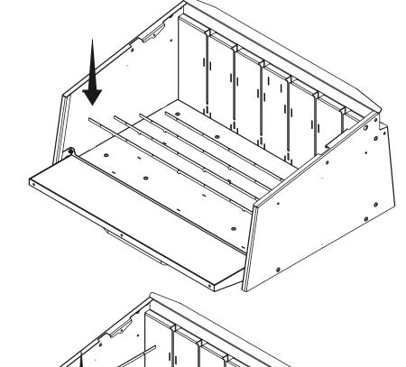
Slot the short lattice parts into the long by aligning the slots in each part and pushing together.
