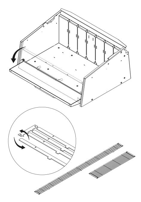
Snap the lattice parts away from the holders by twisting to break the small tab of steel.
